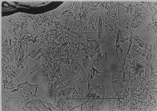
Figure 4. Hexanal droplets in a freeze-dried maltodextrin and hexanal system; this sample was frozen more rapidly and crushed finer than that in Figure 3 (400×)
